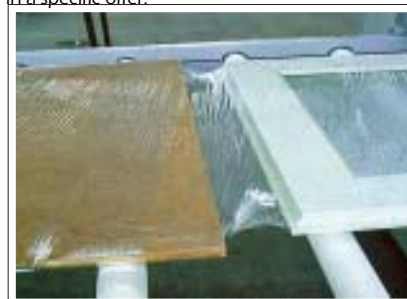
The device for separating the already wrapped goods during continuous wrapping. It allows to increase the wrapping capacity.
